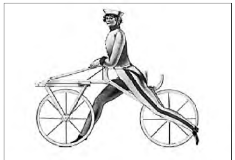
Laufmaschine invented by Baron Karl Drais. From the original patent papers 1817 Scottord Lawrence
